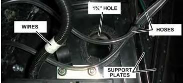
Cut a 1 3/4" hole in the floor to route the cables and wires through. It needs to have a 1/4" clearance for the trim lock. Before you mark or drill any holes, check for support plates or wires under the cab floor.
